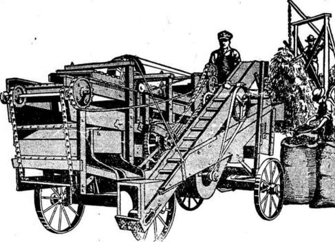
This Picker is the Favorite of Peanut Growers, because it is the Best Machine on the Market. It has larger capacity (300 to 600 bushels per day), operates on less power(six-horse power engine), and
