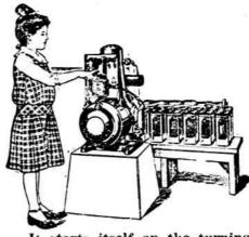
It starts itself on the turning of the switch and stops automatically when the batteries are fully charged.
