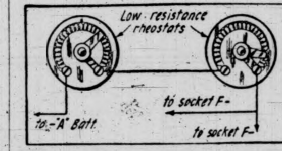
How the Low Resistance Rheostats of a Standard Amplifier Are Connected Up to Be Used With 201-A Vacuum Tubes.
