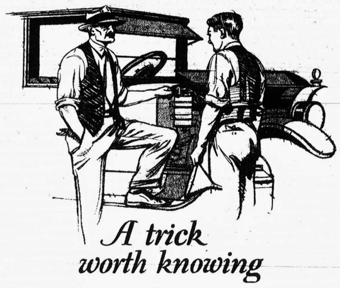
WAIT A MINUTE. You don't need to open up that vacuum tank to fill it after you have run completely out of gas. I'll show you an easier way. Just step on the starter and spin the motor for half a minute or so while I plug this vent with my finger. Your engine will suck the air out of the vacuum tank and fill it with gas for you."
