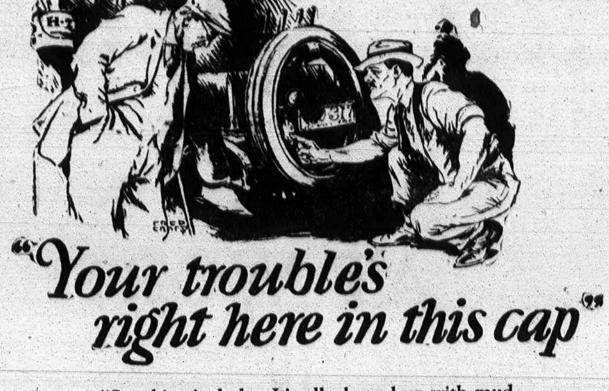
"See this pin hole. It's all plugged up with mud and dust. That hole's the start of your gas feed system. When you use up ten gallons of gas ten gallons of air have to get into your tank. If the air can't get through the cap you'll get a vacuum in your tank and the gas won't flow freely. You'll have trouble sure as shootin' if you don't clean that hole out once in a while."
