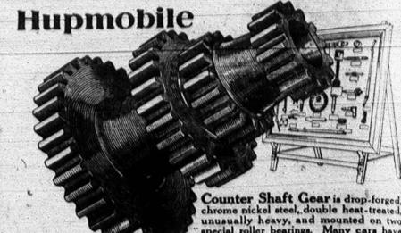
Counter Shaft Gear is drop-forged, chrome nickel steel, double heat-treated, unusually heavy, and mounted on two special roller bearings. Many cars have simply a case-hardened gear of low-carbon steel mounted on plain bushings.
