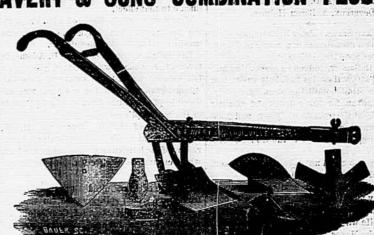
A Complete Turning Plough, with Scraper, Sweep, Shovel, Bull Tongue and Turning Plough.
