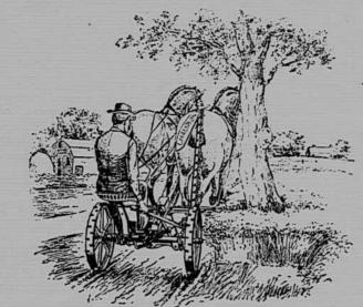
THE CHAMPION MOWER beats the world. Especially adapted for work among trees, stones, ditcnes, &c. No stopping to throw Machine out of gear. You lift the knife without stopping horses or shifting the gear, and go right on mowing.
