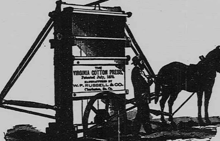
THE ABOVE PRESS IS SO CONSTRUCTED, AND OF SUCH IMMENSE POWER, THAT WITH A SINGLE LEVER ONE MAN CAN PRESS A BALL OF COTTON WEIGHING 500 LBS., OR A HORSE CAN BE HITTED TO THE OPPOSITE SIDE AND PRESS A BALL OF THE SAME SIZE IN ONE MINUTE'S TIME.
