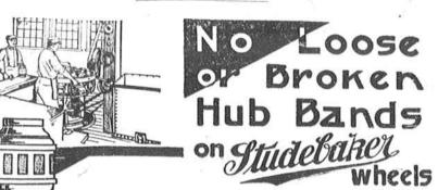
Studebaker hub bands are made of a specially refined iron perfectly adapted for this use. Hub bands are welded by electricity and then shrunk on by hydraulic pressure.
