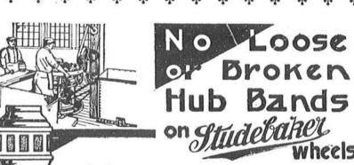
Studebaker hub bands are made of a specially refined fron perfectly adapted for this use. Hub bands are welded by electricity and then shrunk on by hydraulto pressure.
