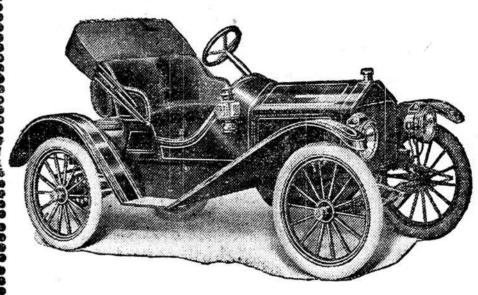
The Meiz 22 Runabout, 2 Passeuger Car is made ap on special features, making this one of the simplest operated cars on the market today. It is gearless with no transmission and no Batteries or Spark Coil to Short Circuit.
