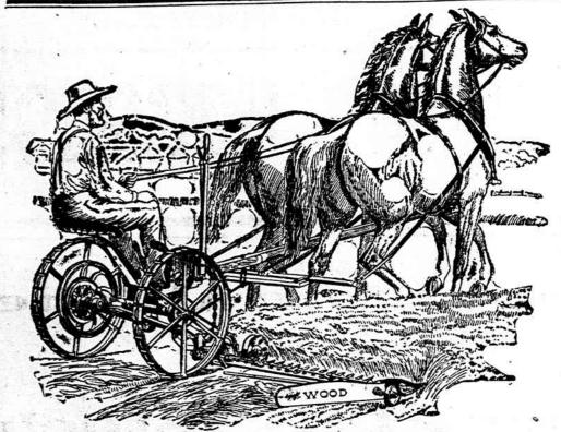
This WALTER A. WOOD MOWER stands out above all others for Light Running, Durability and Simplicity. It runs light because it is roller and ball bearing, and the main frame is cast in one solid piece, therefore there is little wear and tear on machine. : : : : The team is closer to the actual load by several feet than on any other mower made. It cuts the grass uniform, going up or down hill. The driver balances weight of pole. Neck weight on the team cannot
