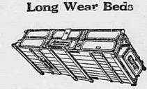
you examine the beds of Thornhill Wagons closely you will see at once the superiority of the construction. The bottoms are re-inforced over front and rear bolsters.
