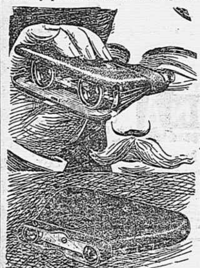
occupies no more room in the pocket. The apparatus is composed of a flat and light frame which has the eye-
