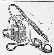
ing it to the point of delivery inside the stylus. Here a flame is presented to ignite the jet, after which frequent pressure on the bulb maintains the flame and controls the temperature of the charring tool. The more rapid the flow of air and gas the greater the heat generated.
