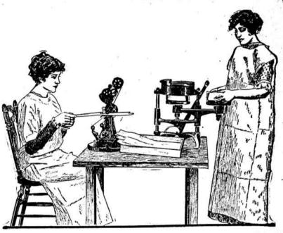
This is the machine we have just installed to launder your collars. It is th? most modern machine made. We dampen the edge so that it folds easily and then mould it in a steam chest so that it has a round, smooth edge and ample space between the outer and inner edges to permit the tie to slip easily.
