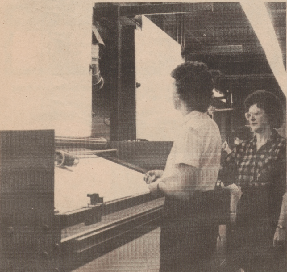
Jackie Ellis and Linda Davis (above) inspect a roll of fabric as it passes across new inspection equipment in Plant No. 1. The material handling equipment enables cloth room personnel to virtually eliminate manual handling of huge cloth rolls. Richard Bowie (right) enters data on a package put up directly into the computer. He records weight, style, yardage, bale numbers and other data necessary to facilitate inventory and shipping.
