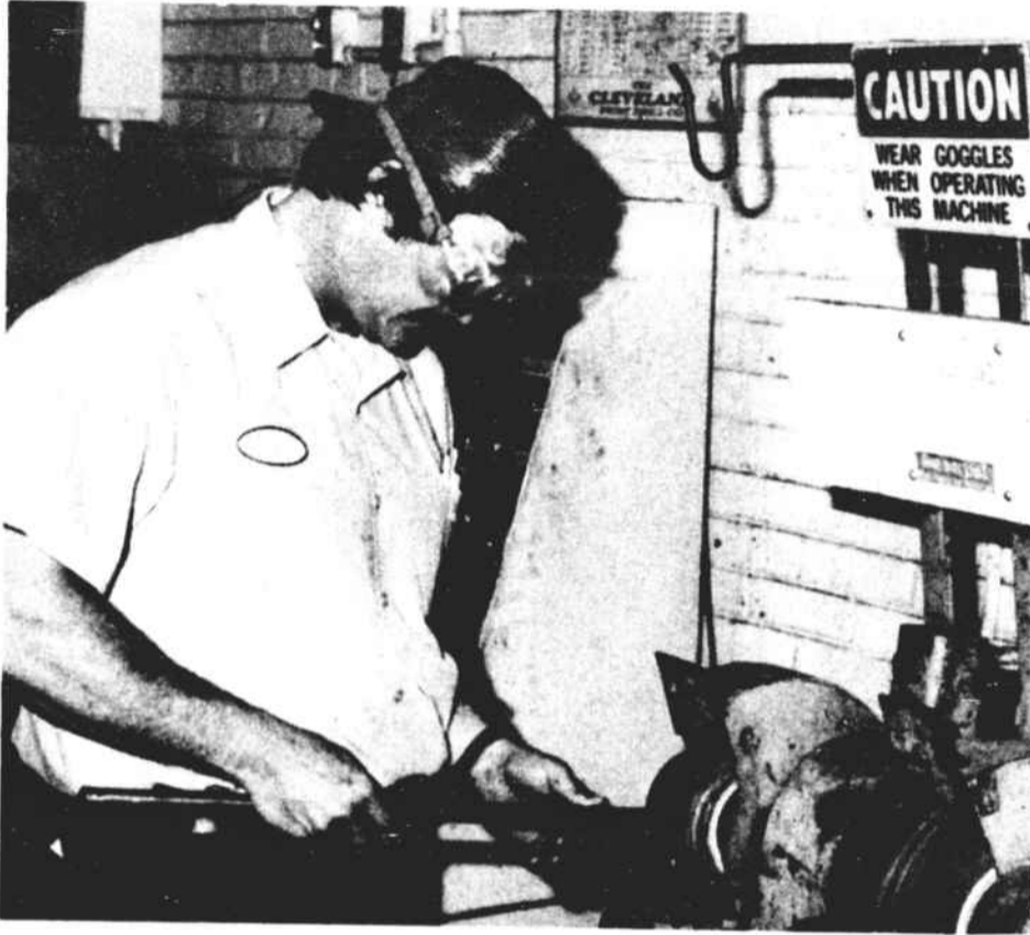
Marshall Vaughan observes all safety precautions in operating grinders in the Clinton Mills Maintenance Department. Grinders cause flying chips and sparks which are particularly hazardous to the eyes and other parts of the face. Wheels occasionally shatter during operation, presenting even greater danger unless safety precautions are taken.
