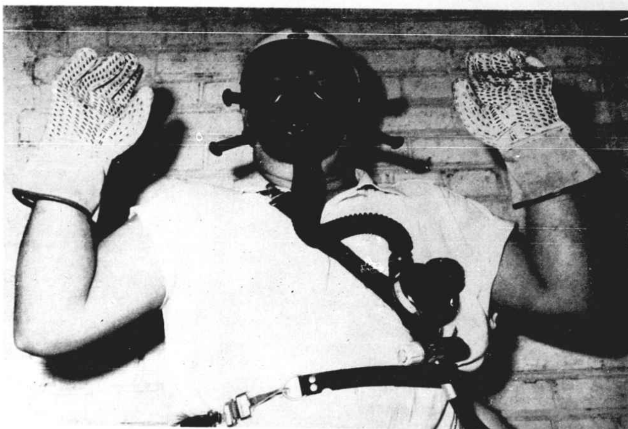
NOT A MAN FROM MARS BUT FROM OUR MILLS —This is some of the new safety equipment in use at Clinton-Lydia Mills, and which employees now are receiving instruction in its use. It consists of an air mask for breathing in smoke-filled rooms, or rooms with any foreign contamination in the air. Also shown are a protective helmet and wire-strengthened protective gloves.
