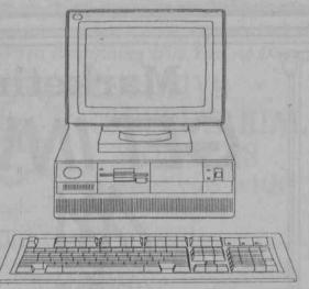
IBM PS/2 Model 50Z (1.44 MB 3.5" floppy drive, 30 MB hard disk, 1 MB active memory, Intel 80286 chip, Microchannel architecture, Zero wait states, VGA color monitor, Mouse) List price: \$4099.00, USC students: \$2679.25
