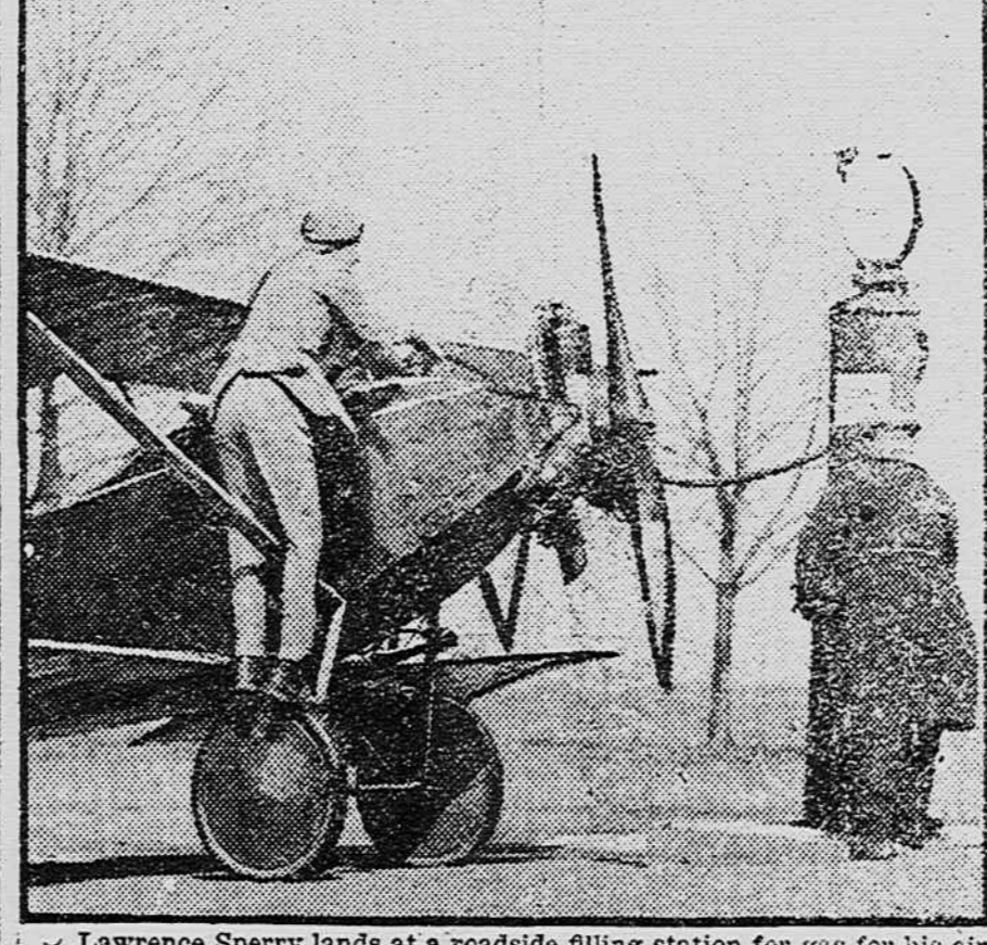
Lawrence Sperry lands at a roadside filling station for gas for his air flivver. It weighs only 600 pounds and can land in an ordinary street.
