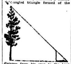
distance from his eyes to the base of the tree, fro " his eyes to the top of the tree, and of the height of the tree itself. As the base and the altitude of this triangle are equal, it follows that the height of the tree is the same as the distance from his eyes to Its base.
