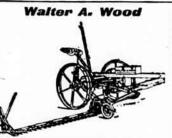
because it is the only mower that has genuine underdraft, "floating" frame and uniform tilt, the three big mower features no farmer should be without if he values his own time or his teams' strength, and wants the machine that does most work the easiest.
