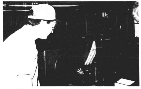
Lydia Shop employees have devised a movable plexi-glass shield for the metal lathe to prevent metal chips from striking the operator.
