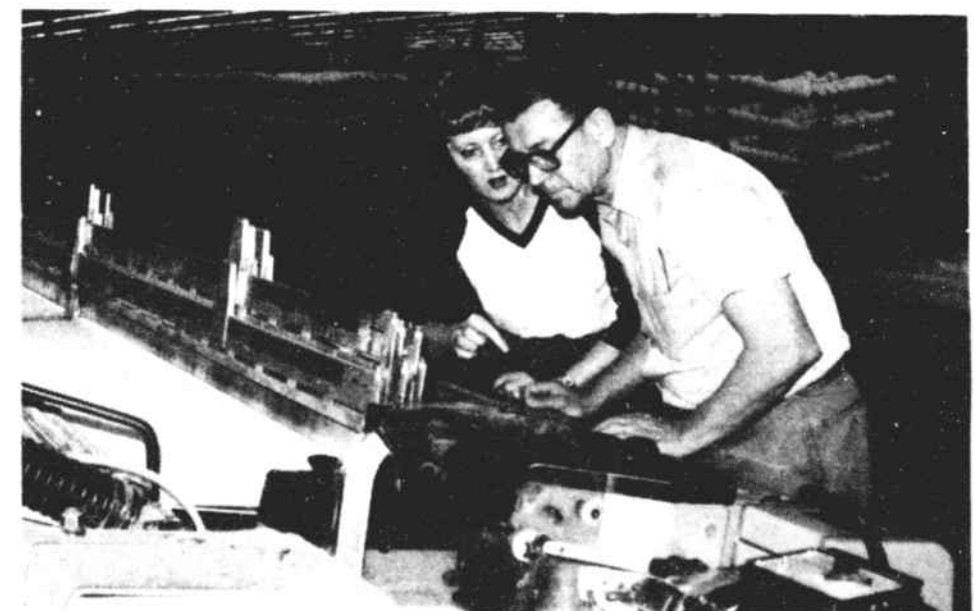
THIS IS THE WAY IT'S DONE —Allie Campbell instructs Prue Waters in proper weaving practices on the new machines. Prue is training on a Sulzer PS4000 which has a maximum reed spread of 157 1/2" and can produce three 48" panels simultaneously at 325 picks per minute.
